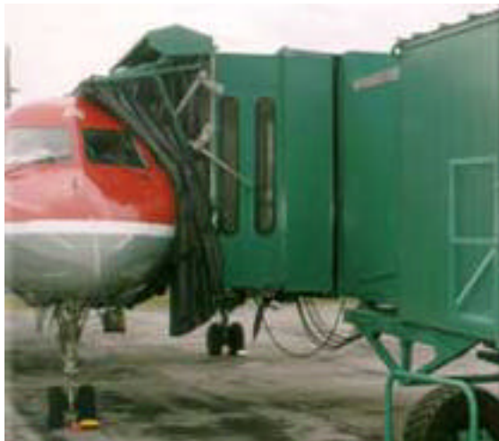
Fig. 1 Low Loading Bridge for Small Aircraft
